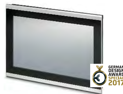
Configurable panel PC with Intel® Atom™ E3845 technology
